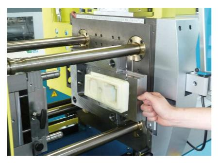
The cassette mould (with 3D-printed cavity insert) can be exchanged in a few simple steps.
