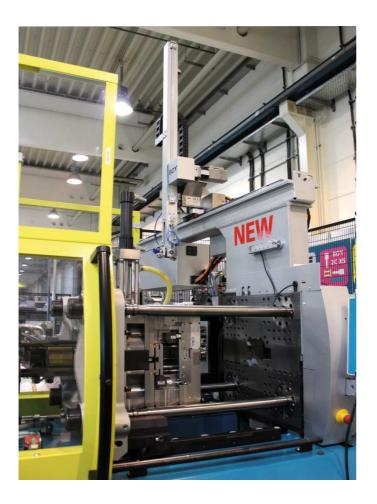
The new servo-motor-driven linear handling BOY LR5 with an attractive priceperformance ratio is a complete new development of the manufacturer of injection moulding machines up to 1,000 kN clamping force.
