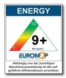
These guidelines focus on the most environmentally friendly and resource-saving operation of injection moulding From **perfor**machines. mance class 1 (worst assessment) to class 10 with an energy consumption of only 250 Watt per processed kg of plastic, fixed efficiency classes have been created which are manufacturer-independent in terms of machine technology. Depending on the machine size and its equipment, the BOY E-series has a Euromap classification of 9+
