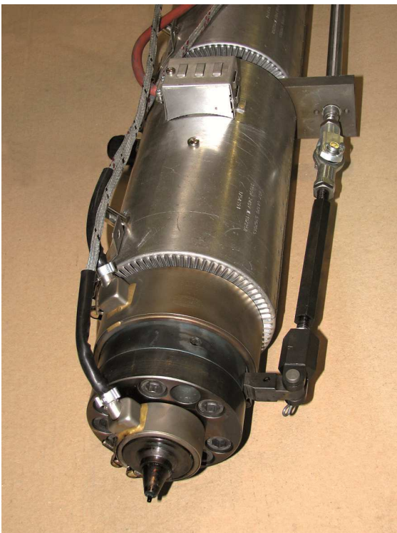
Photos:> Plasticizing cylinder with BC nozzle
