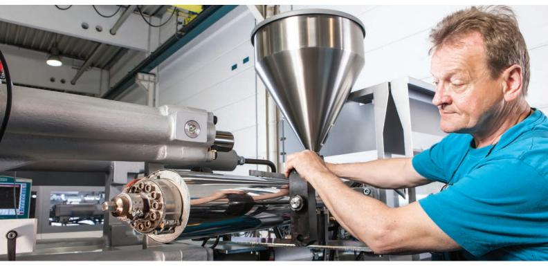
As an option, the high wear-resistant Econplast units are available for all BOY injection moulding machines, from a screw diameter of 18 mm upward.
