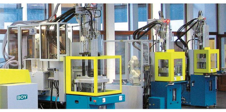
Also all insert moulding machines from BOY are available in the technical centre for individual series of tests and test injections.
