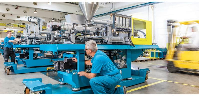
The highly modern flexible, flow manufacturing machines are transported to the ergonomically equipped assembly stations on variable carriages.
