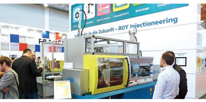
A complete manufacturing system: Injection moulding machine BOY 100 E with four-axis industrial robot handling LR 5, as well as a protective enclosure conforming to CE.
