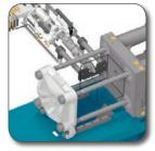
Horizontal mounting at the side of the mould (horizontal L - Position)
