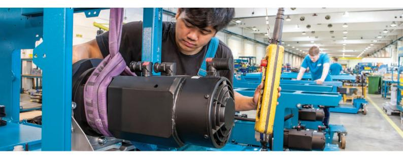
The efficient servo-drive is installed in the BOY injection moulding machines since 2008.
