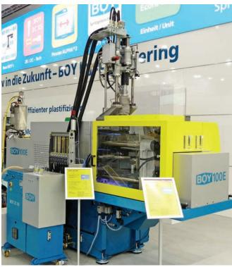
The machine controls communicate with each other via special interfaces (such as EM 67) and ensure a smooth sequence of the injection moulding cycle. So a multi-point connection of injection units on a bigger injection molding machine is possible.
