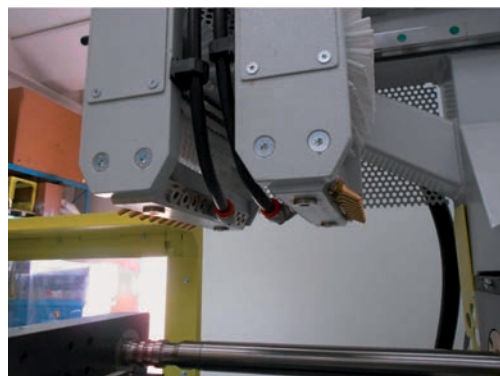
Spraying device beneath the brush rollers
