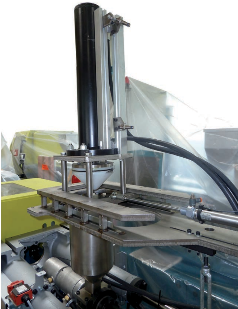
Hydraulic driven stuffing unit on top of a plasticising unit
