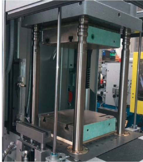
BOY 35 E VV with heating platens (mould fixing by T-slots) and core lifting device.
