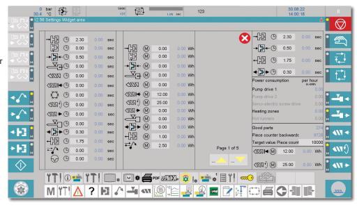
With the modified visualisation of the user interface, users of previous BOY-machine controls won't have any problems in getting around with the new Procan ALPHA ® 6, as the basic programming concept has been maintained.
