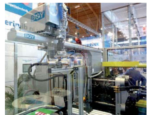
Production of ICE model railway housings on a BOY 100 E.
