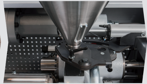
Electrically driven material hopper / feeder for an easier refilling / assembly
