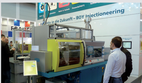
Production cell with CE-compliant safety housing
